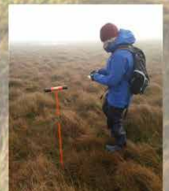
Surveying for the depth and extent of upland peat.
